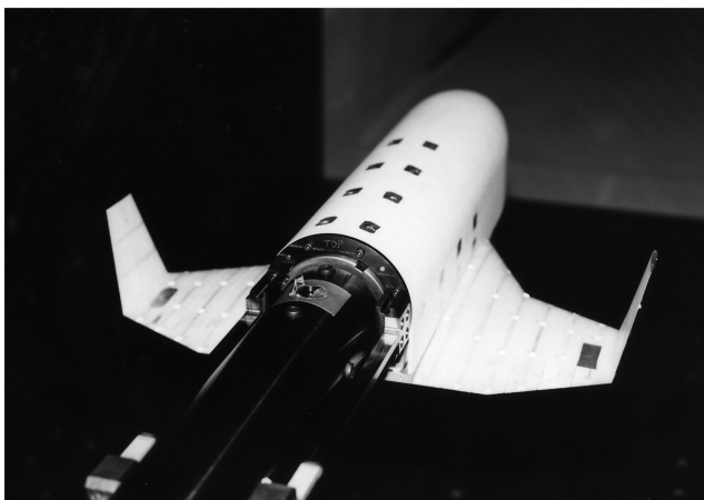
Fig. 9 Wind tunnel model for launching configuration.
